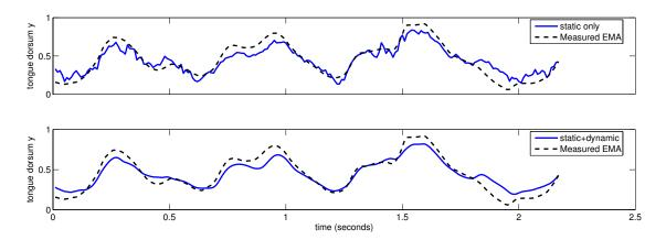
Figure 3: Comparing the MLP-equivalent (only static features) and the full Trajectory MDN (dynamic features and the MLPG algorithm) for the utterance "The speech symposium might begin on Monday." The trajectory MDN output is smoother and closer in nature to the real trajectory, and more accurate (e.g. around 0.5 and 1.5s).
